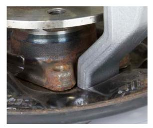
The press feet get access to the small surfaces close to the bearing, pressing on the knuckle behind the brake shield.
