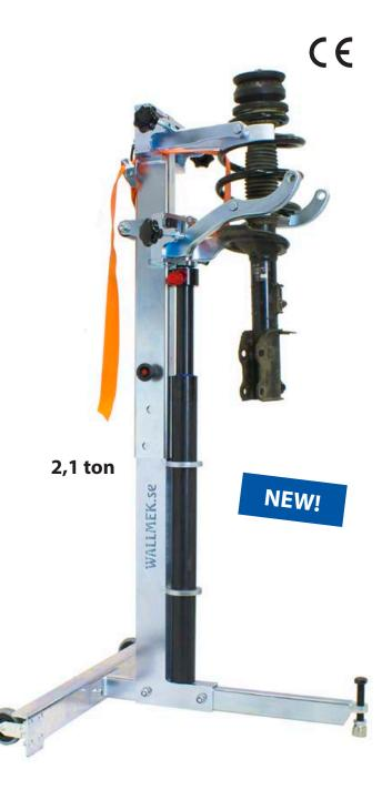
This function allows the operator to compress the spring and split the shock absorber unit from the wheel spindle/knuckle directly on the car. The same function can also be used to unload the lower control arm to its "driving" position when working with ball-joints or sway bars. With pressure on the spring instead of the lower plate, the lower plate rubber can be replaced in just minutes.
