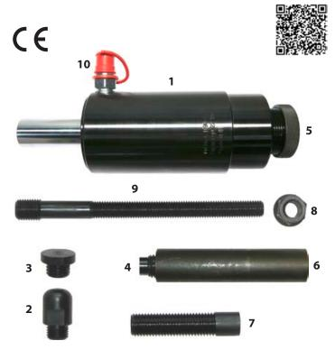
Can be used with all of our passenger car tools and carriage beams M10-M22 with the proper adaptor. The cylinder's hydraulic pressure can be combined with punching force when using the punching socket 1086-6. For example when pressing a rusted axle shaft. Weight: 4,7 kg. Stroke: 70 mm. **Automatic return.**
