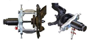
Bolted on bearings are often used in aluminium knuckles but also frequently used in steel knuckles. The small tolerance in combination with long guiding in to the knuckle causes huge problems after some years when removing the bearing. To avoid damaging and to avoid removing the wheel knuckle
