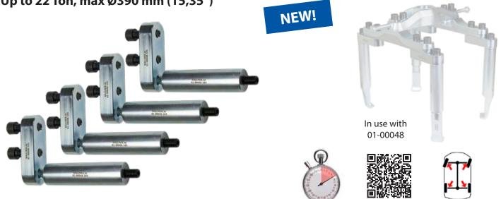
This add on set is used with 01-00048 brake disc/rotor puller. Presses disc/rotors up to Ø 390 mm (15,35") without destroying the wheel bearings even when the disc/rotor is over 330 mm.
